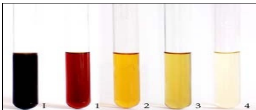
Plate.3 Color of effluent fractions after column chromatography (I- Effluent showing initial color; 1, 2, 3, 4 - Effluent fractions showing color after passing through the packed biomass in series of four columns)
