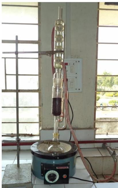
**Fig.1** Soxhlet apparatus
