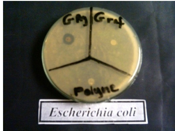
Figure.4 The antibacterial activity of PAN, Cs-g-PAN copolymer and Cs-g-PAN/Ag nanocomposite against E. coli
