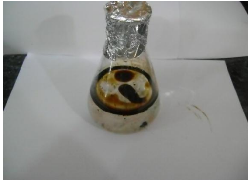
Fig.5 Biodegradation of crude oil by mixed culture of A. niger and A. fumigates after 28 day incubation
