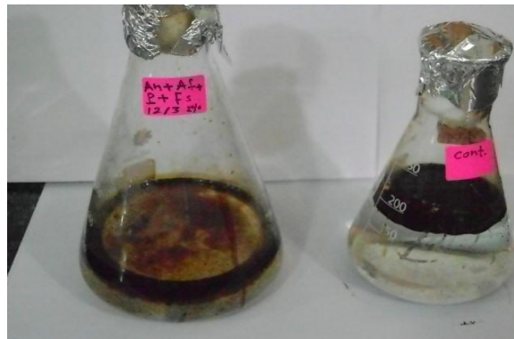
Fig.7 Biodegradation of crude oil by A. niger , A. fumigatus , F. solani and P. funiculosum after 28 day incubation
