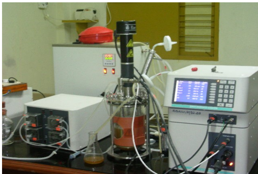
Figure.2 Biosurfactant Production by Bacillus sp. CS14 using a lab scale Fermentor
