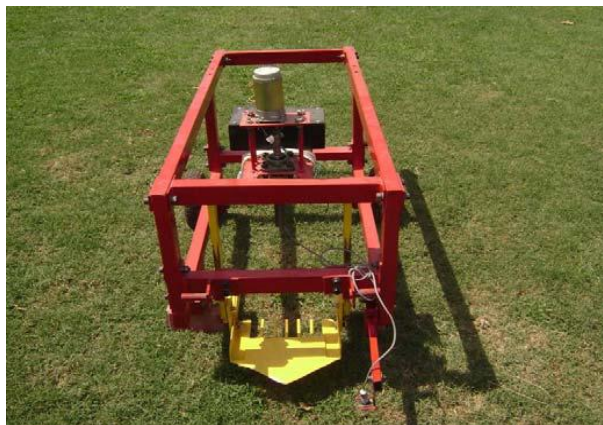
Fig.2 Head of onion harvester including control depth system
