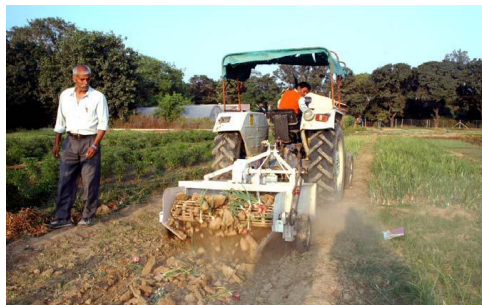
Fig.2 Head of onion harvester including control depth system
