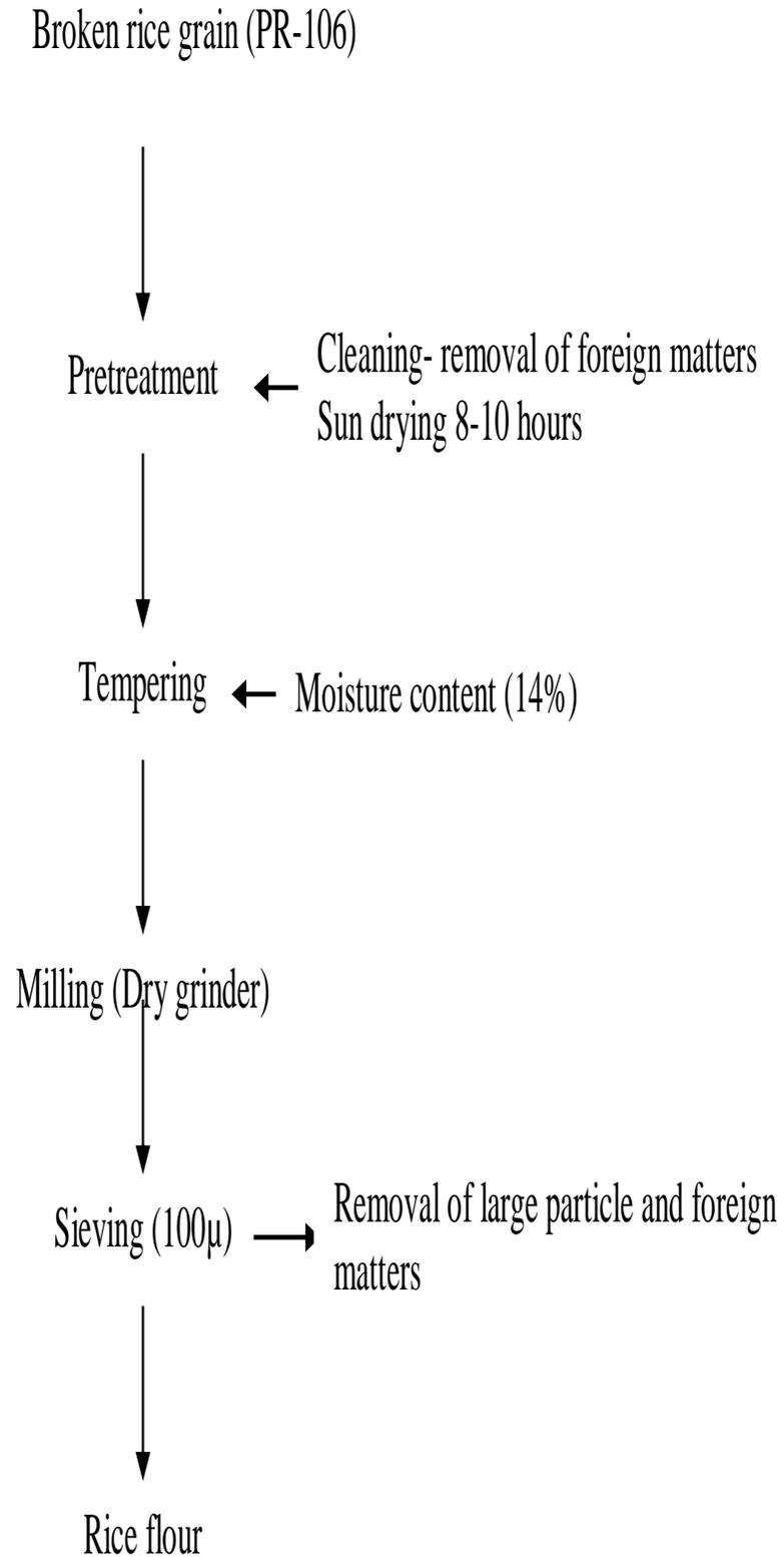
**Fig.2** Flow diagram for isolation and purification of starch from broken rice grains
