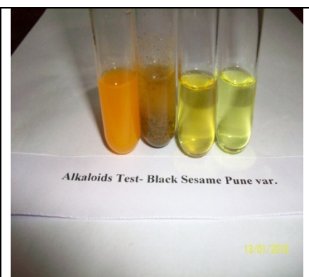
Fig.3 Brown precipitate indicates presence of alkaloids in black sesame seeds. The extracts were in sequence of ME, WE, MR, CR. ME and WE showed the presence of alkaloids.
