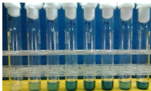
Figure 2. Phosphomolybdenum method showed that Camellia sinensis leave extract showed the antioxidant activity of 12mg/gram where B-Control, S1, S2, S3, S4 and S5 are ascorbic acid standards. The T1 and T2 are test samples
