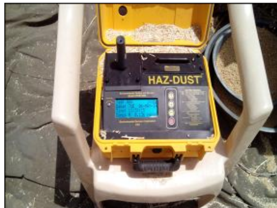
Fig.3 Dust concentration measurement in threshing
