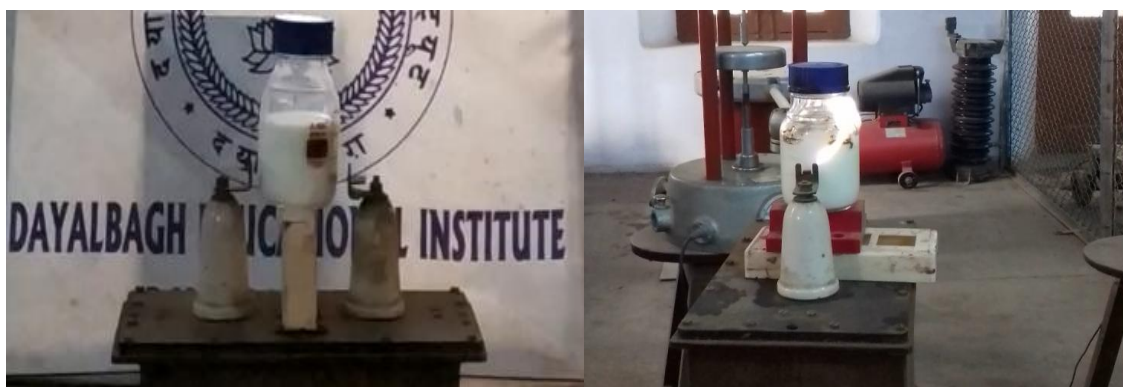
Fig.3 Treating milk with HVEF
