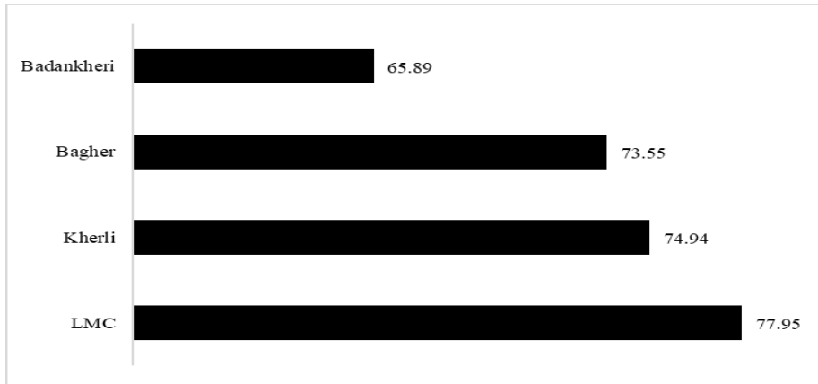
Figure.2 Water conveyance efficiency ( E_c ) for LMC and its selected minors
