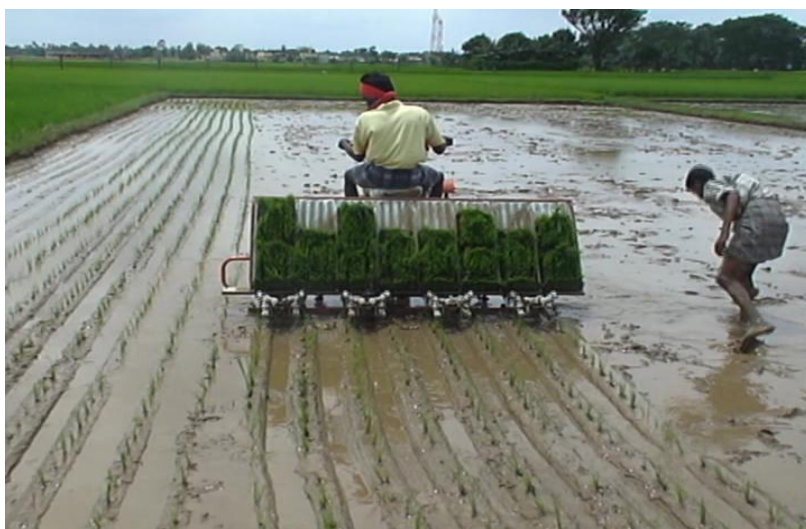
Fig.1 Self-propelled eight row paddy transplanter
