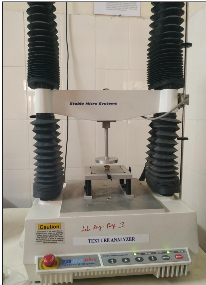
Plate 4 Experimental set up for testing of rupture force of aonla stone
