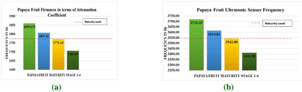
Figure.7(a) Ultrasonic sensor data for frequency (b) computed value of attenuation coefficient of fig 6(a)
