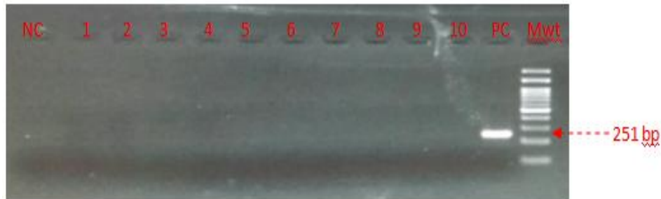
Fig.6 Agarose gel electrophoretogram showing specificity of the gyrB PCR primer ( S. epidermidis )
