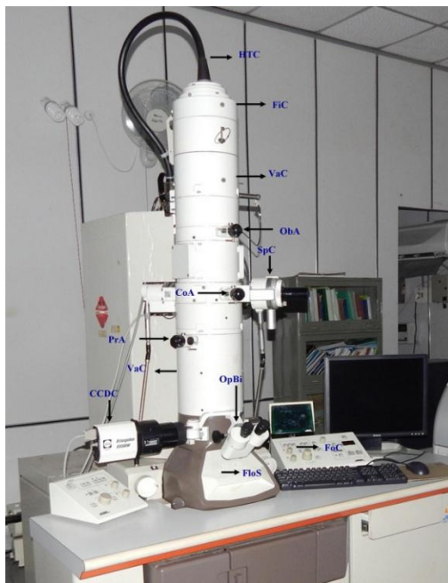
Fig.1 Transmission electron microscope (JEOL-JEM 1011, EM Laboratory, G.B. Pant University of Agriculture and Technology, Pantnagar) showing High tension cable (HTC), Filament chamber (FiC), Vacuum chamber (VaC), Objective aperture (ObA), Specimen chamber (SpC), Condenser aperture (CoA), Projector aperture (PrA), Charge-coupled device Camera (CCDC), Optical binoculars (OpBi), Fluorescent screen (FloS) and Focusing control (FoC)
