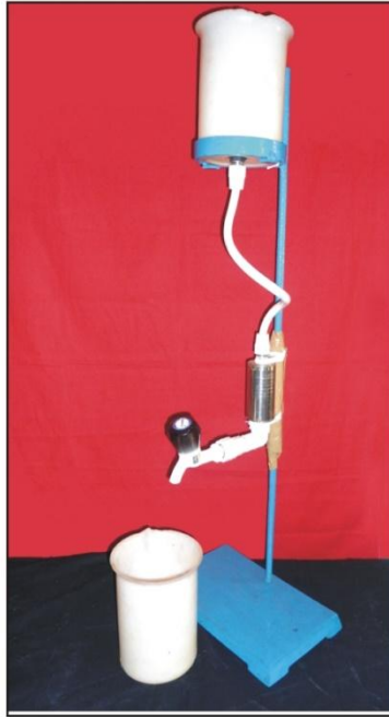
Plate 1. The magnetic device used to magnetize irrigation waters
