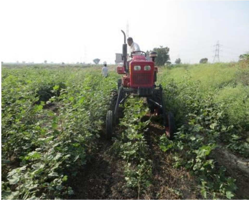
Plate.1 Performance evaluation of small tractor operated intercultivator cum fertilizer applicator in cotton crop
