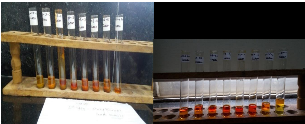
Fig.4 Chilli and curry samples showing positive results for the Presence of Sudan by colour test
