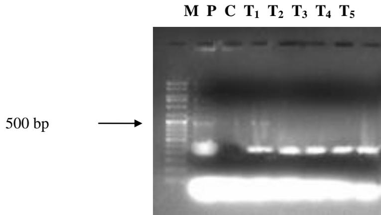
**B: Confirmation of presence/integration of transgene (*hpt*) into the genome of lettuce using polymerase chain reaction**
