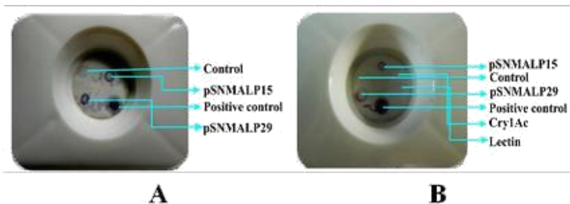
Fig.3 A. Detection of Cry2B antigen through rapidot on NC-membrane cassette, B. Cross reactivity test of developed scFv antibodies against different different antigens
