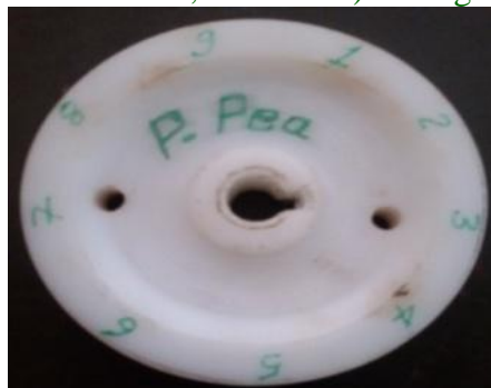
Fig.1 A fabricated view of seed metering wheel for a manually operated multi-crop planter (Developed in SHUATS, Allahabad) for Pigeon pea seeds
