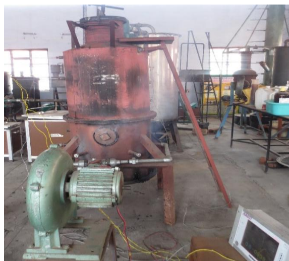
Fig.1 Designed updraft gasifier
