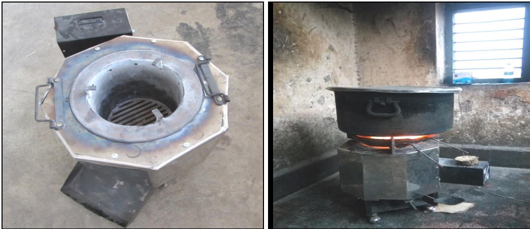
Figure.4 Developed community cook stove in operation
