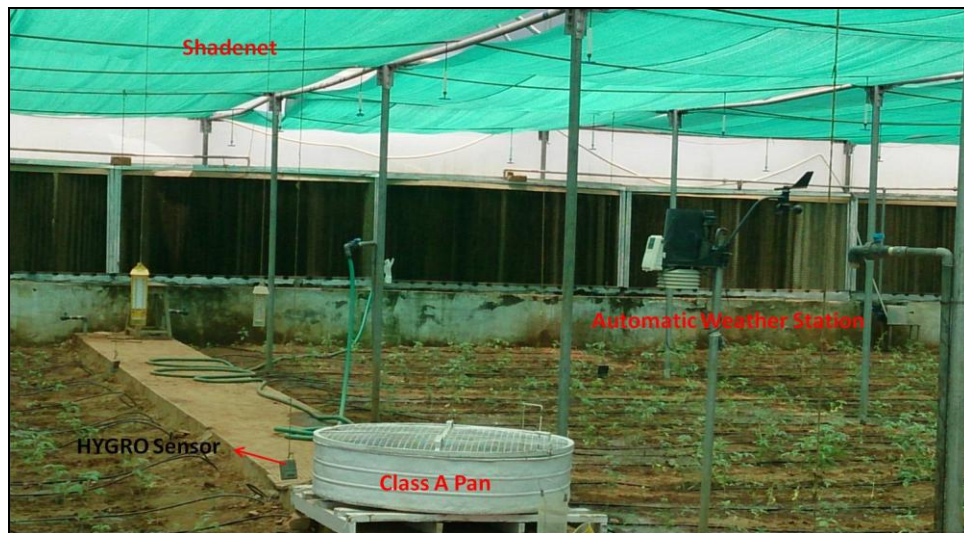
Fig.4 Automatic weather station, Class A Pan and HYGRO sensor installed in Polyhouse
