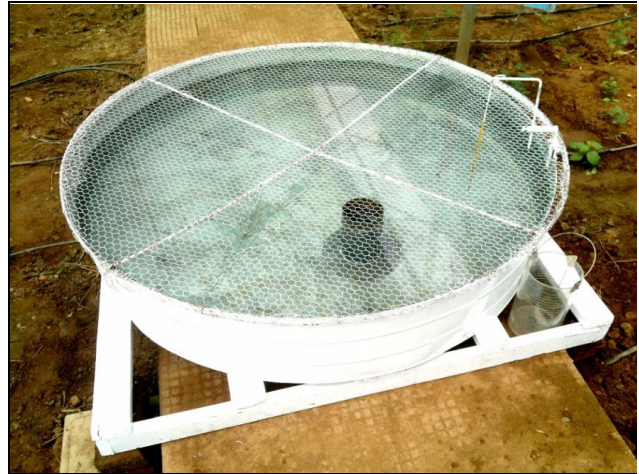
Fig.4 Automatic weather station, Class A Pan and HYGRO sensor installed in Polyhouse
