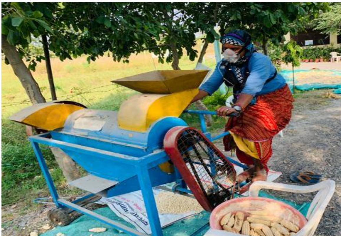
Fig.4 Shelling operationby Pedal-operated maize de-husker sheller used in the study
