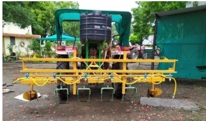
Fig.5 Developed tractor drawn Inter-cultivator cum sprayer with cotton hoe assembly
