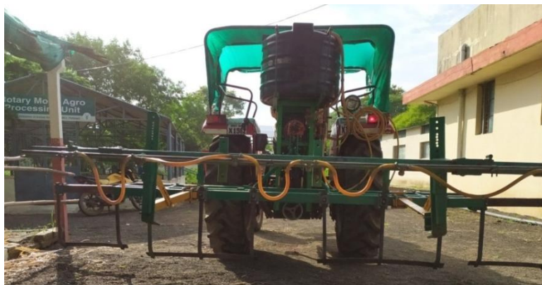
Fig.5 Developed tractor drawn Inter-cultivator cum sprayer with cotton hoe assembly
